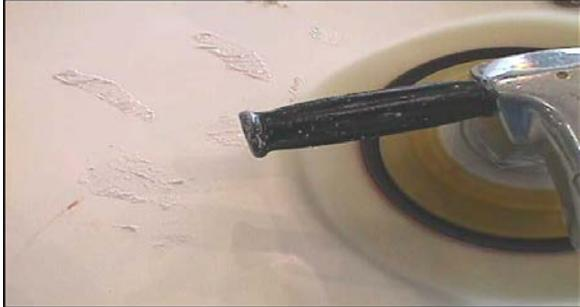
Buff the area with a mild compound to remove the 600-800 grit scratches. Repeat until the area is free of sanding scratches. Do not burn or over buff the area. This can discolor or remove all of the gel. Polish to a deep shine with a wax or glaze.
