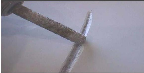
Prep the area removing all of the damaged gel coat. Keep the repair as small as possible. Prep the damaged area with 220 grit sand paper. Sand down any rough edges. A Dremel tool or die grinder can also be used to prep the damaged area. Cracks must be ground out prior to applying patch paste.
