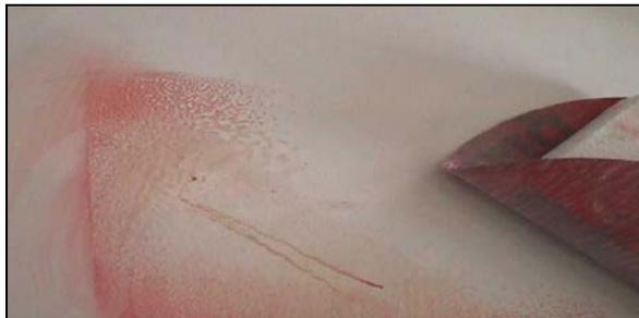
Mark the repair area with a grease pencil. This prevents over sanding. Sand the patch with a 220 grit sand paper. Sand only as much as necessary to remove the excess material and or the grease pencil's color. Keep the block or sander flat to prevent a wavy patch. Repeat process with 400 and 600 grit paper.
